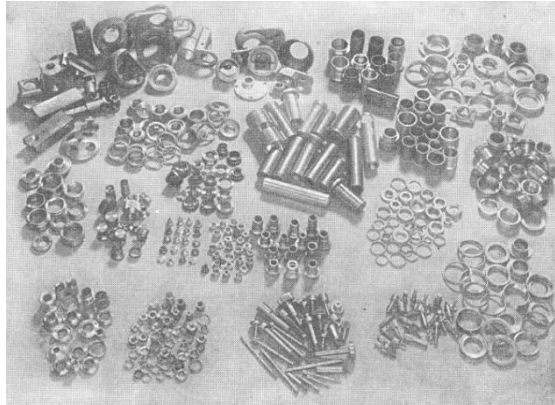
Fig. 2. An example of grouping parts of a rotary shape [8]
