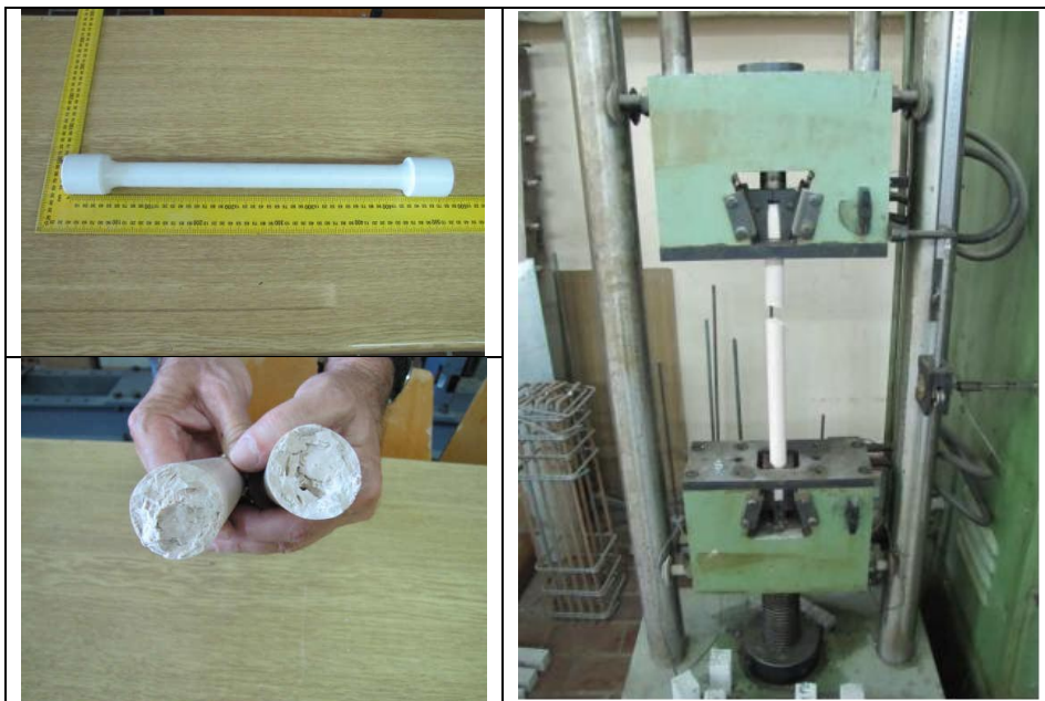
Fig. 2. Characteristic shape of samples for tension testing, sample during testing and cross section of the sample after testing
