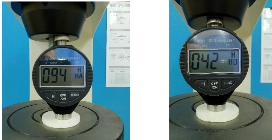
Fig. 5. Device for measuring the hardness of TPU parts
