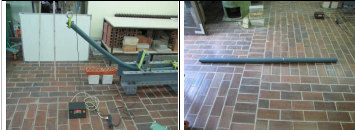
Fig. 5. Bending testing of circular cross-section columns until failure and reversible deformations on the sample after testing
