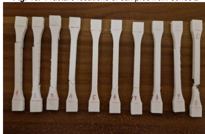
Fig. 14. Fracture locations of samples from series 3
