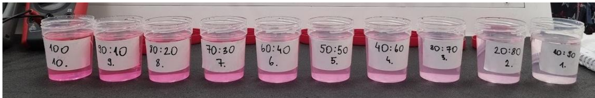
Fig. 3. Coolant samples of 100 ml with different volume fractions of distilled water and antifreeze
