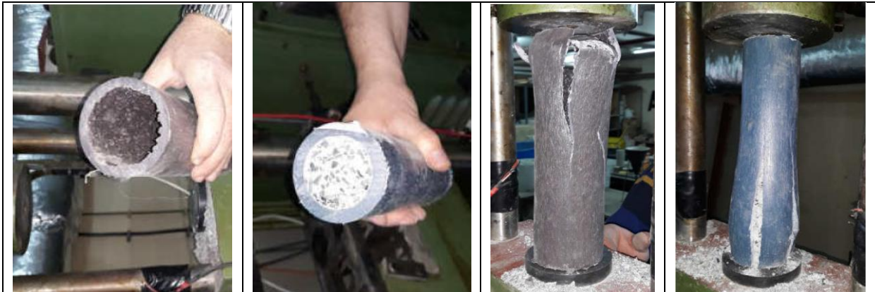
Fig. 3. Samples during testing: circular cross-section and columns after testing (hollow and full)
