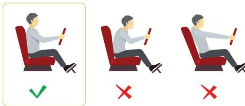
Fig 1. Correct / Incorrect driver posture [2]
