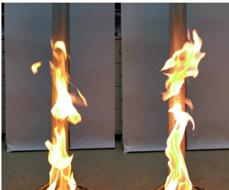
Fig. 5. Two frames for the same HRR illustrating the pulsating nature of the turbulent methane flame
