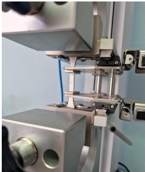
Fig. 8. Specimen placed in the jaws of the tensile tester machine
