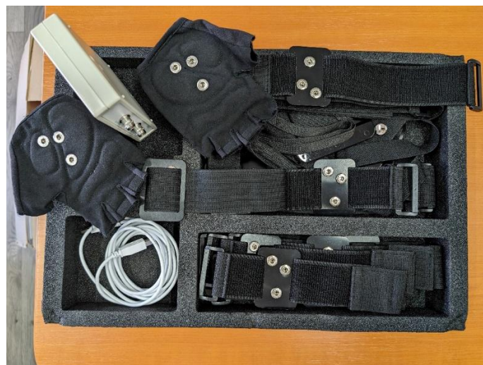
Fig. 4. Elastic bands used for attaching sensors to the driver
